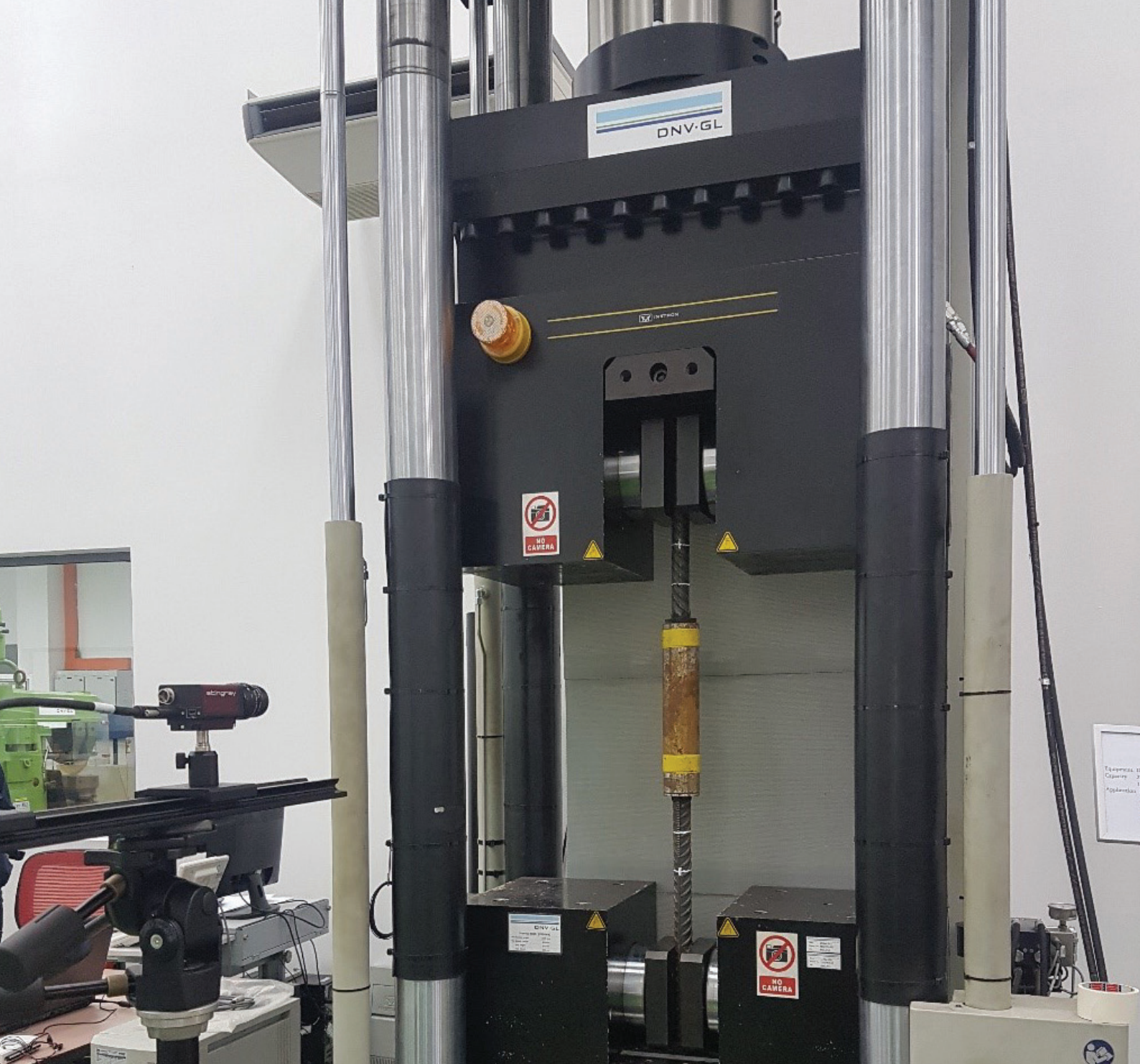
Testing performed at DNV-GL's Laboratory with the 2500kN Dynamic UTM and Video Extensometer. Photo courtesy of DNV – GL Singapore Pte Ltd
