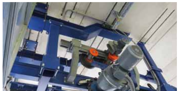
Thanks to the HALFEN Channels, components with a very high load distribution can be precisely positioned and readjusted at any time. Anchor and mounting channels were used here.
