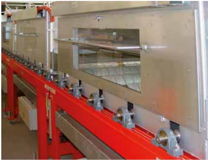
Easy installation and adjustment of bearing blocks using Halfen Mounting channels and T-bolts
