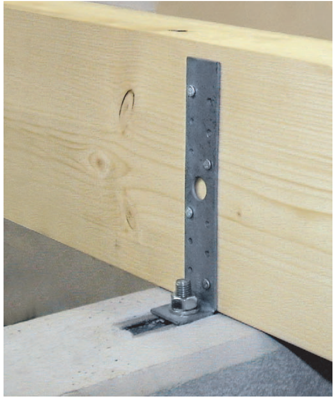
Connecting construction timbers to concrete using Anchor channel and a Halfen HNA Timber fixing strap type WN 185
