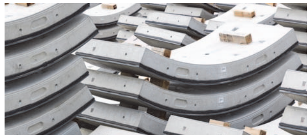
Curved Halfen Anchor channels in tunnel segments
